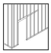
Measure up from the floor "door height+1-3/4 in." to the centerline of the track. Leave at least 2 in. from the end of the track to the side of the door opening. Use a level to level the track and mark screw holes. Drill 1/4 in. pilot holes.
