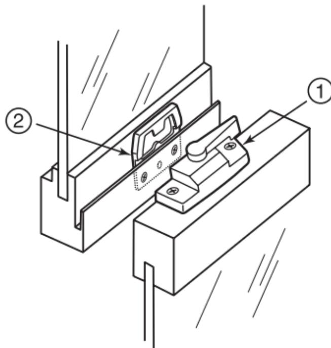
Check new latch and keeper for proper alignment and hole spacings on window frame. Mount latch (1) in existing holes or mark new location and pre-drill 3/32" new holes. Install and set to locked position. Align keeper (2) with cam, pre-drill holes (if needed) and install.
