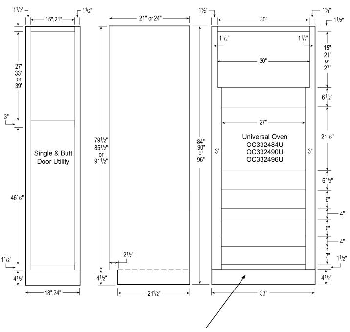
NOTE: 96" TALL CABINETS ARE SUPPLIED WITH LOOSE TOE KICK BOX (EXPOSED SIDES REQUIRE TSK96)
