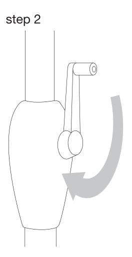
1. Turn the crank handle clockwise until the umbrella is fully opened.
