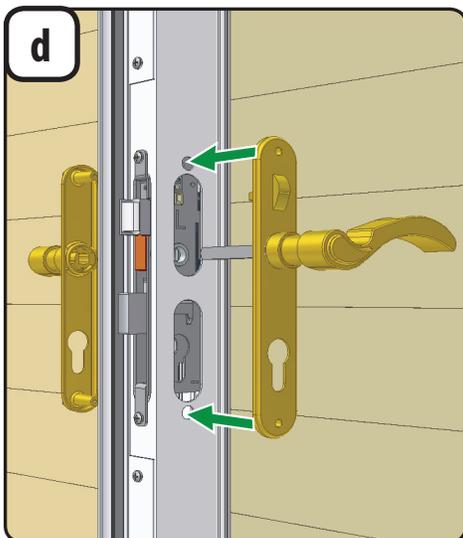
1. With handle levers held horizontal, install both handle assemblies onto door. Spindle will pass through square hole in lock case and into other handle. Attach trim plates together using two 1 1/2" pan head screws.
