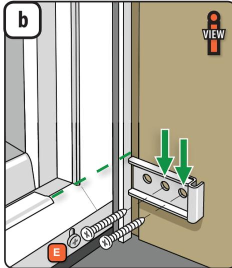
1. Position base from installation kit onto door jamb by touching front of base to back of hinge rail (or as close as possible), and align top of base with top of retainer channel. Mark the hole locations on door jamb.
