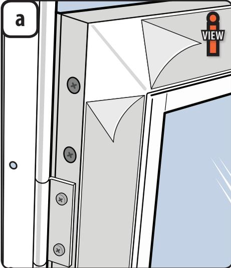
1. If applicable, start at the mitered corners and remove the clear protective tape from both the interior and exterior of door frame.
