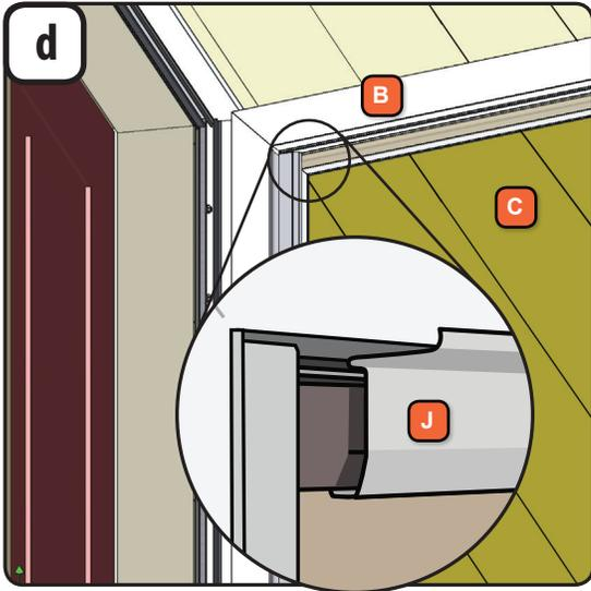
1. Center glass panel (C) in bottom of door frame (B) and carefully tilt it forward into opening in frame.
