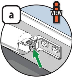
1. Open the door and then let it close. Note the speed at which the door closes.
