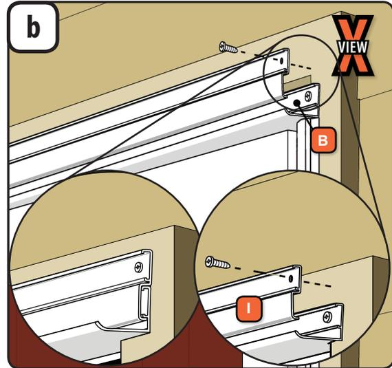
1. If a plug was installed in the middle hole, you will need to install the rain cap extender (I).
