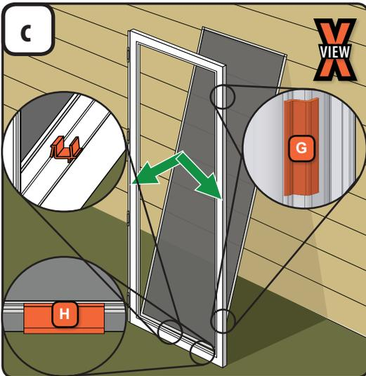
1. Supporting weight of door by door frame, remove door from carton and remove tape holding insect screen to door frame.
