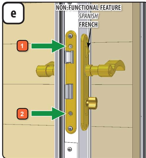
1. Install lock case trim plate onto lock case and fasten with one 5/8" screw. Do not overtighten.
