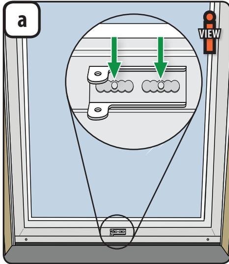
1. Attach closer door bracket to the door through the two pre-drilled holes using two #12 x 5/8" screws.
