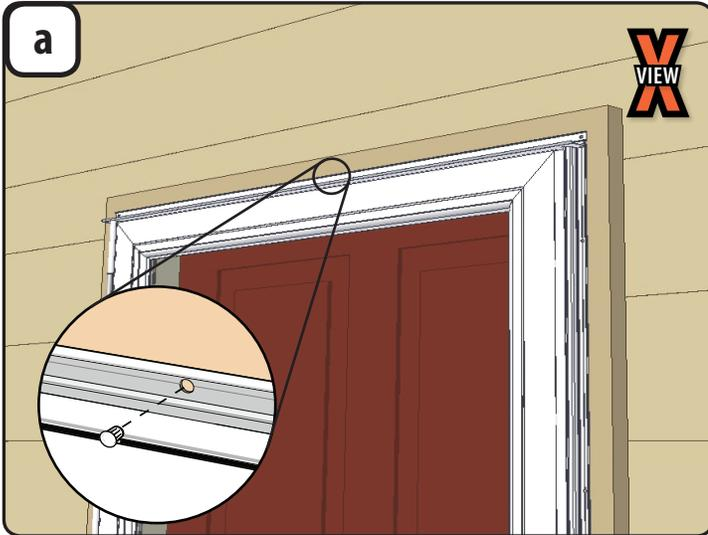
1. Look at the center hole of the rain cap. If the mounting surface can be seen in the entire hole, proceed to **step a2**. If the mounting surface cannot be seen in the entire hole, or if there is space above the rain cap, then completely insert the 3/16" plug into the middle hole, then proceed to **step b**.
