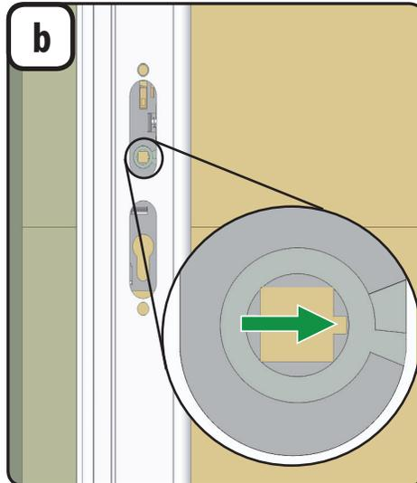
1. Look into handle holes on door to make sure lock case is oriented properly. Notch in square spindle hole should be facing away from glass panel.
