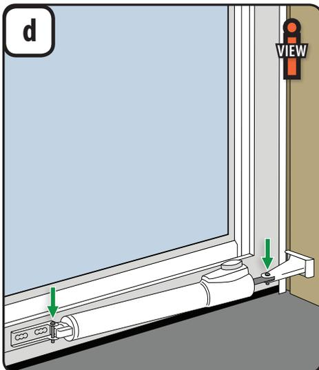
1. Pin bump closer in place using the short pin in the jamb bracket arm and the long pin in the door bracket.
