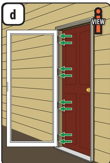
1. Using 1/8" drill bit, drill holes in door jamb through holes in hinge rail.
