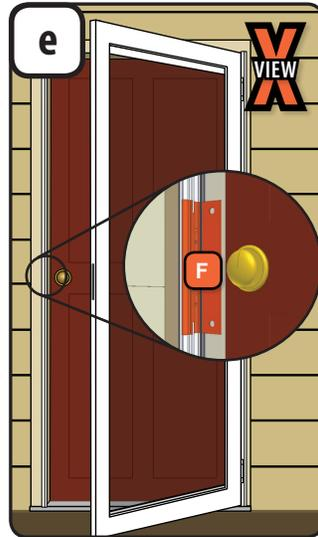
1. Grasp handle clip (F) and pull away from latch rail to remove.
