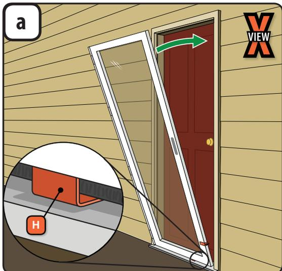
1. Set bottom of door centered in opening. Make sure orange bottom spacer (H) is sitting on door sill.
