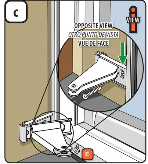
1. Attach the arm from the installation kit to the base by inserting the tabs on the arm into the slots in the base. Fasten with a 2" screw from the installation kit.
