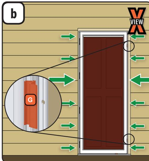
1. While holding door in position, use 1/8" drill bit from closer kit (O) to drill a hole in the mounting surface through two pre-drilled holes (indicated above with extra-large green arrows).
