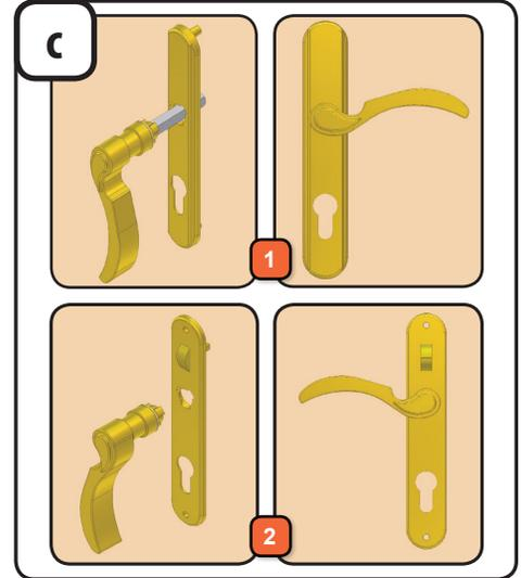
1. Insert handle into outside trim plate (with Andersen logo) with lever pointing down and rotate handle to secure it.
