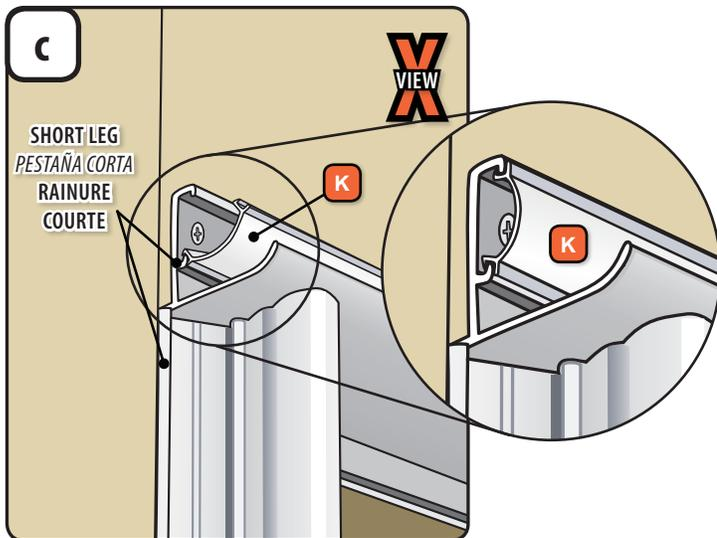
1. Lock leg of screw cover (K) into short leg of rain cap screw track. Press on other leg to snap it into long leg of track. Make sure screw cover snaps into screw track along the entire length of the rain cap.
