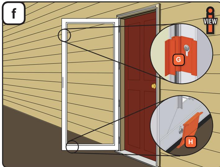
1. Remove spacer clips (G) by loosening but not removing screws.
