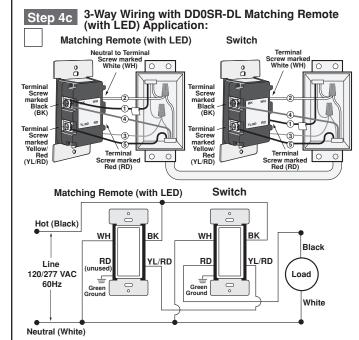
**NOTE:** The switch **must** be installed in a wall box that has a Load connection. The matching remote must be installed in a wall box with a Line Hot connection and a Neutral connection. A Neutral wire to the matching remote needs to be connected as shown.
