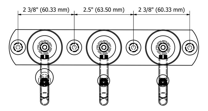
Step2: Attach unit to Mounting Surface.
