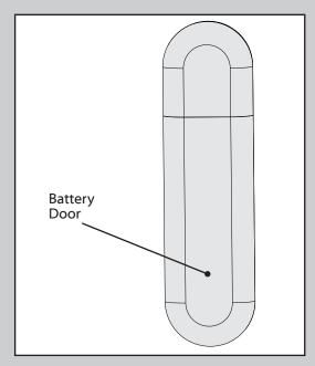
To access the battery compartment, remove the battery door from the transmitter assembly. The battery should be installed with the positive (+) side up. Replace with a CR2032 battery when necessary.
