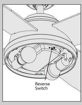
To switch the direction of air flow, move the reverse switch to the opposite position. You will need to remove the glass to do so.
