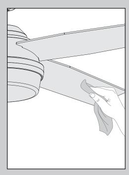
When cleaning the fan, use soft brushes or cloths to prevent scratching. Cleaning products may damage the finishes.
