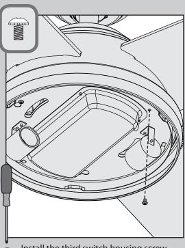
Install the third switch housing screw.
