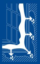
Other influences, which will have an effect on the integrity of your sealing joints, will be the normal subsidence, which occurs in buildings. The drying and cracking of mastics used to seal joints and the expansion and contraction of wooden or concrete floors, may cause the tiles to de-laminate or move from their original position.
