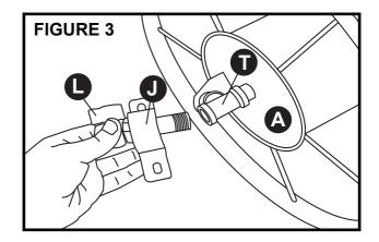
3. Spool Assembly: Screw galvanized tee (T) onto spool. Insert brass swivel (L) thru U-bushing (J) and screw into galvanized tee (T) on the spool (A). Tighten using a wrench. **Figure 3**
