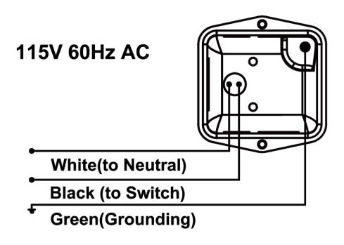
**Figure 2**: Wiring Diagram - Single speed. 115-volt connection. for ILG8SF18S(APB-18B), ILG8SF30S(APB-30B), ILG8SF36S(APB-36B)
