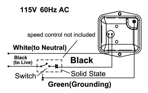
Figure 1: Wiring Diagram - Speed Controllable. 115-volt connection.
