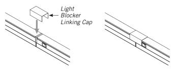
Install Cap <u>after</u> lights have been hung and you've confirmed that they work properly. Be sure your lights are aligned and have no gap between, then remove the red tape plastic and place the cap down firmly on the top surface of the light, centered on the connection between the two lights.
