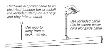
When suspending single, stand-alone SlimLights, each light will need an AC power cord connected to the top AC power input. When suspending multiple lights linked together, one AC power cord can power up to 10 lights max (3.3 amps, 320 watts total).
