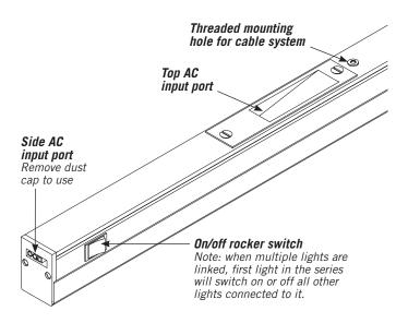
Turn on/off the SlimLight with the rocker switch, or connect the power cable to an outlet or circuit controlled by a wall switch.
