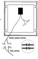
TIP: To increase the power of the fan, additional solar panels may be added, using the easy-connect clips.
