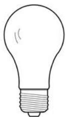
Light Bulb (Maximum 60 watt Medium Base Incandescent Bulb or CFL equivalent)
