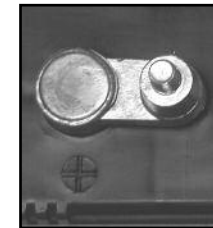
POSITIVE POST HAS LARGER DIAMETER
