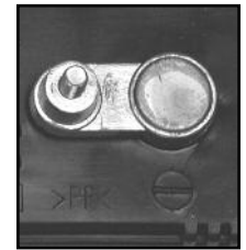
NEGATIVE POST HAS SMALLER DIAMETER
