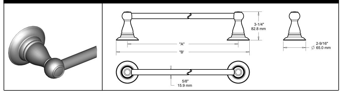
MATERIALS: Post - Zinc Die Cast Bar - Steel Wall Plate - Steel, Zinc Plated
