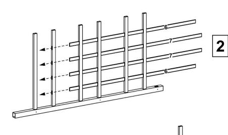
Insert two 63" vertical slats (part 6) through outer holes of center cross rails and into bottom cross rail. Insert two 66" vertical slats (part 7) through inner holes of center cross rails and into bottom cross rail.
