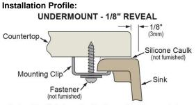
Designed to affix to the underside of any solid surface countertop.
