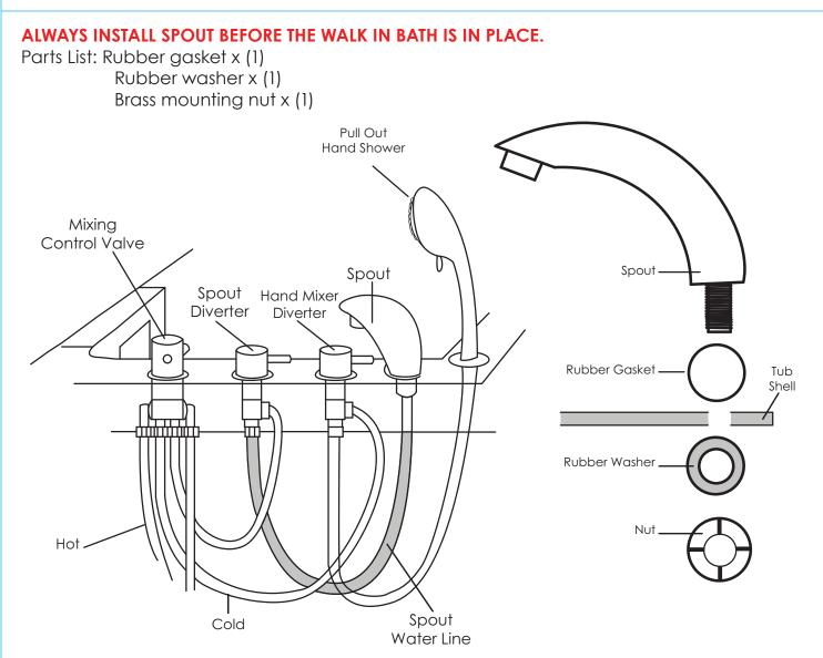
To Install the supplied spout, first place the rubber gasket on the bottom of the spout and make sure it is properly seated in its groove. Put the spout in through the hole in the tub shell (shown in the drawing above). Install the rubber washer and then the brass mounting nut. Locate the water line from the spout diverter and connect it to the threading on the bottom of the spout. Tighten all fittings and check for leaks.
