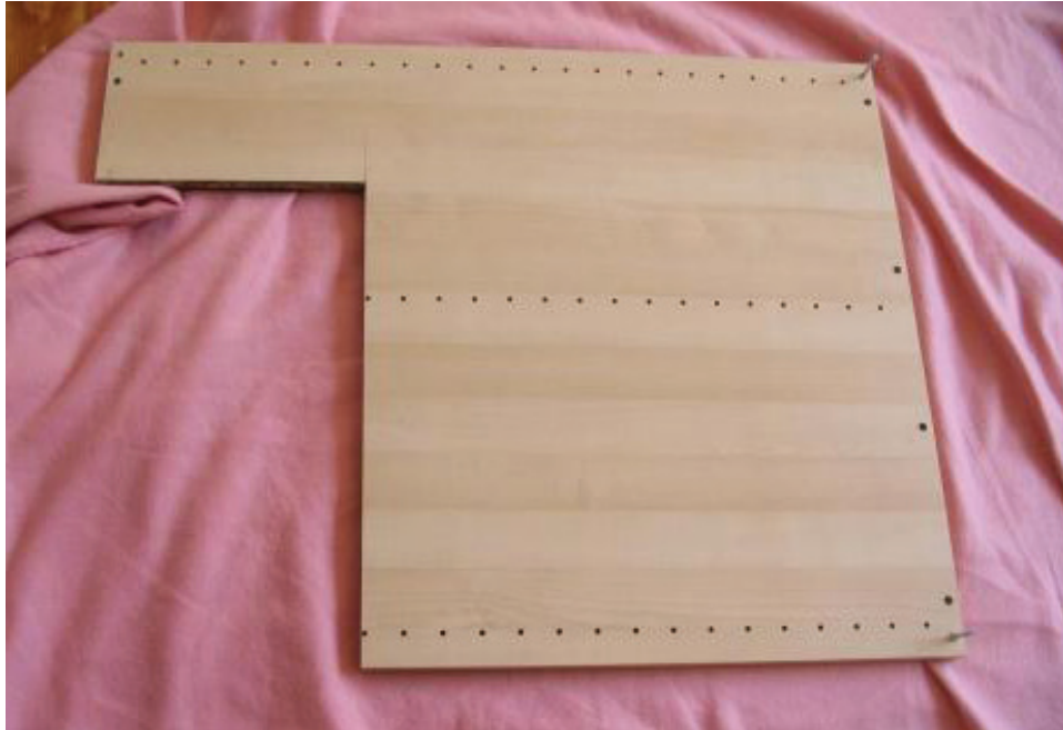
[Above]: Make the cuts to the cabinet. Here, a table saw was used.
