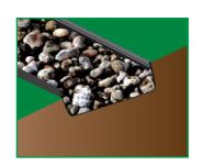
Last to secure from any lifting, backfill Channel Guard with rock or any other landscaping material.
