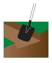
Using a square point shovel begin digging a trench the width of the Channel Guard to desired area. Keep center of trench level to insure proper installation. When installing the Channel Guard for downspout diverter applications make sure the trench is sloped away from the foundation for proper drainage.
