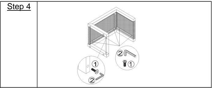
Align Side Support Bar(A) to Side Panel(C), Top Panel(B), and Base Support Bar(D). Attach Side Support Bar(A) to Side Panel(C), Top Panel(B) using Bolts(①) with Allen Key(②) as shown above.
