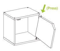
Orient door properly as shown and align bottom pin. Press on spring loaded top pin and insert.
