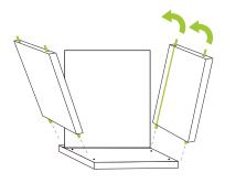
First fit backer board in groove, then arrange vertical zBoard with grooves facing backer board as shown.
