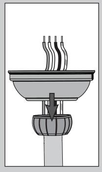
Put the wires and downrod through the canopy. Let the canopy sit loosely on top of the fan.
