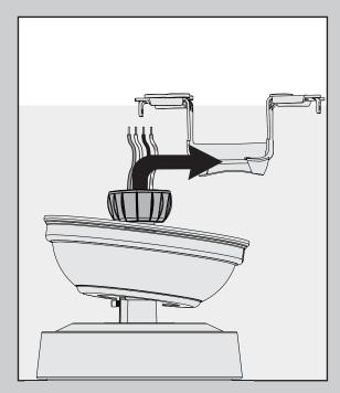
DO NOT PICK THE FAN UP BY THE **CANOPY OR WIRES.** Place the downrod ball into the slot in the ceiling bracket.
