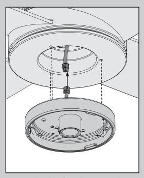
Connect the plugs from the upper and lower switch housings. Make sure to line up the colored markings on the connectors. Lift the lower switch housing until its screw holes are aligned with the screw holes in the upper switch housing.
