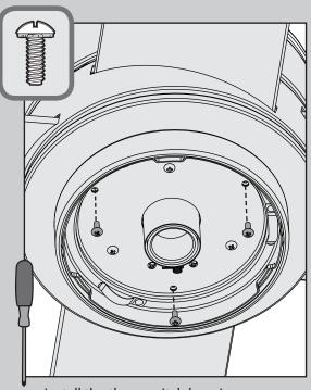
Install the three switch housing screws, found in the ≡ hardware bag. Tighten all three screws.
