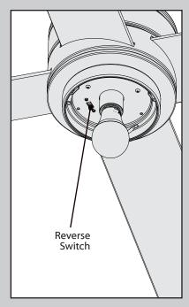
Changing the direction of air flow - move the reverse switch to the opposite position. You will need to remove the glass to do so.
