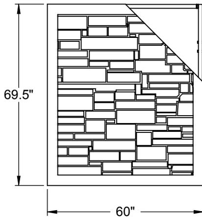
Gate is reinforced with a 1.5" galvanized steel box tube.
