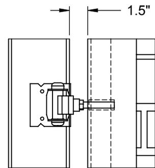
Gate hinge threads into the upper and lower inserts in the gate metal frame leaving about 1.5" from the edge of the gate to the gate post.
