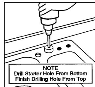
4. Identify fixture hole locations. Drill a starter hole from reverse side. Working from the top side as illustrated, position a hole saw on the starter hole and drill to complete the fixture hole. Attach faucet, drain, and accessories according to manufacturer's instructions.
