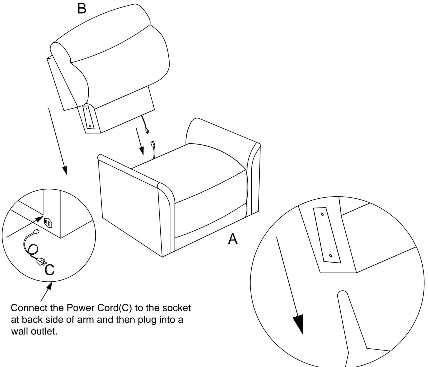
Connect the Power Cord(C) to the socket at back side of arm and then plug into a wall outlet.
