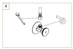
Apply pipe tape onto threads of water supplies. Use wrench when tightening the hose connection. Do not overtighten.
