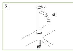
IMPORTANT: After installation is complete, remove aerator and turn on water supply and allow both hot and cold water to run for at least one minute each. While water is running check for leaks; make adjustments if necessary. Reinstall aerator. Your new faucet is now ready for use.
