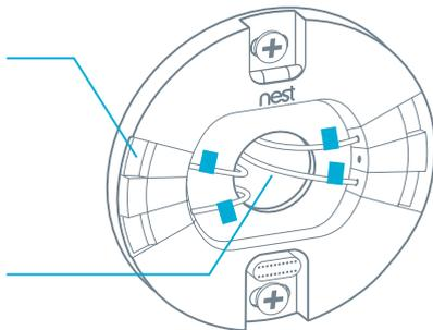
After all the wires are securely connected, push them down to make sure they're flush with the base.
