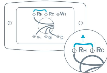
**IMPORTANT:** If you have Rh and Rc wires, you have a dual transformer system. The Nest Thermostat E is not compatible with dual transformer systems, but you may be able to use the 3rd generation Nest Learning Thermostat.
