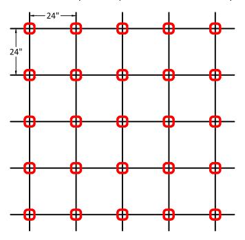
If rebar spacing is greater than 12", place chair at **every** rebar crossing. If rebar spacing is 12" or less, place chair at **every other** rebar crossing.
