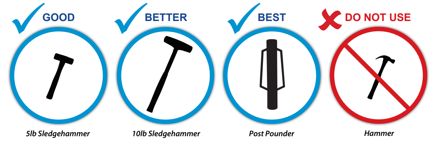
5lb Sledgehammer 10lb Sledgehammer Post Pounder Hammer Purchase post pounder at any hardware store or go to: www.wambamfence.com . Post pounders cost roughly $25 to $30 at Hardware Store (or rental stores often have for rent). Inside diameter of post pounder should be 3" diameter minimum.
