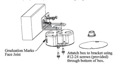
**Caution:** Disconnect power supply. Use RACO® supplied screws only (except 8-32 screws for light fixtures). Connector installation through inside of the box. Maximum NM cable 10-3 with ground.
