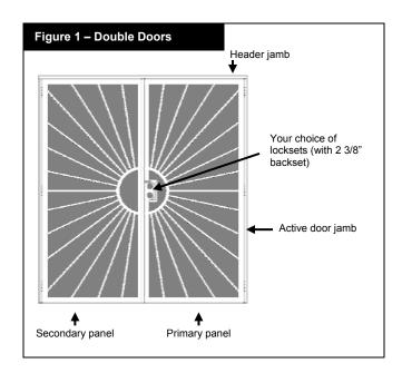
**Step 1** – Attach your choice of locksets (with 2 3/8" backset). Fully extend the lock bolts into the "Locked" position.
