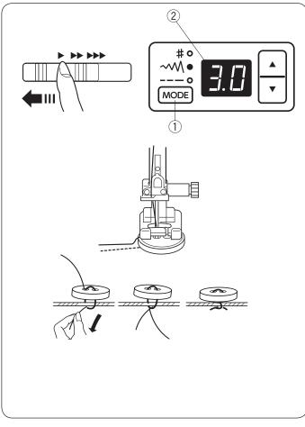
Lower the feed dog (refer to page 13). Set the speed control slider at a slower speed.
