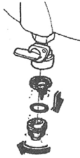
Fuel Filter Element Removal
