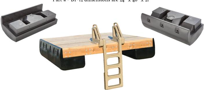
TechStar Bumper Floats are a unique combination of dock bumper and flotation. Designed to run the length of your dock on both sides, these floats will comfortably float a dock 8-feet wide. For docks 10 to 12 feet wide we recommend one row of center floats and for docks 14 to 16 feet wide we recommend 2 rows of center floats.
