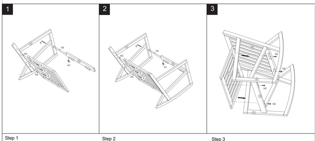
Attached (A) to (B),(D) and using (H3) to put on the hole.(E),(H1) tighten by (H4)
