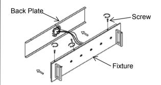
Attach fixture to the back plate, using screws provided.
