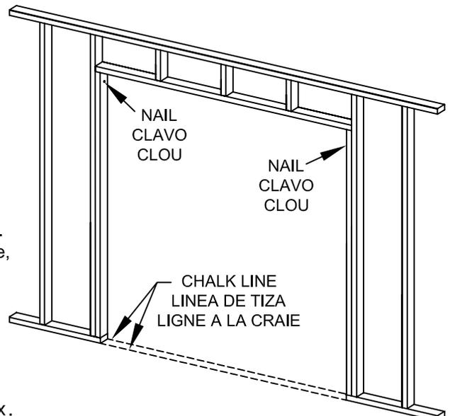
**4** Slip slots in Frame Header End Plates over nails in rough studs. LEVEL HEADER. Set nails and drive nails through remaining holes in end plates. (If you have the 2/6" (761mm) or Universal Frame and using another size door, see cutting instructions on page 4.)
