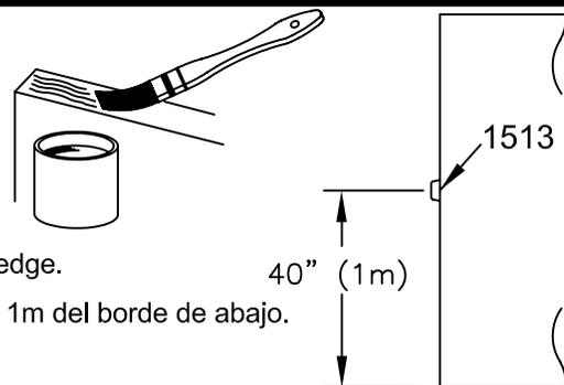
**8** Fasten 1513 Bumper on back edge of door 40" (1m) from bottom edge.
