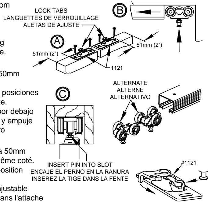
**10 Install** finished jambs, split header and casing as shown. Fasten split header on 1121 lock lever side with screws for future door removal or adjustment. **DO NOT USE JAMBS WITH DADO'S.**
