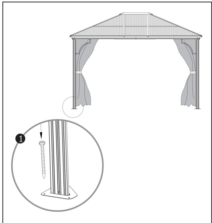
In order to firmly secure your structure to the ground you need to use screws, in accordance to the surface your product will be installed upon. Install the screws in the pre-drilled holes of the bases (K) of the shelter. Screws are not included. This step is mandatory for the warranty to apply since this is a permanent structure.
