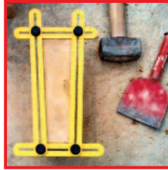
Axed Shape for Bullseyes and Arches
