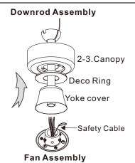
2-3. As shown above, insert yoke cover, deco ring, canopy onto downrod.
