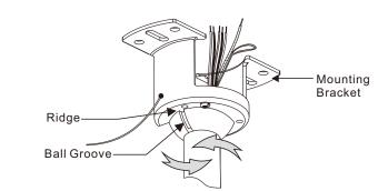
3-2. Rotate fan so that the groove on the ball engages the ridge in the mounting bracket.
