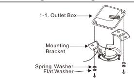
1-1. Install mounting bracket to outlet box on ceiling by using screws included with the outlet box and washers from the hardware bag.
