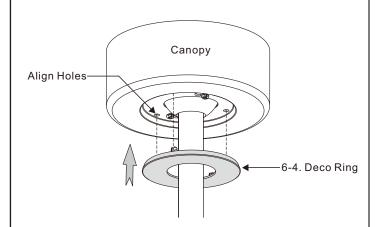
6-4. Push deco ring up to canopy, align holes on canopy with ribs on deco ring, and push "snap-in".
