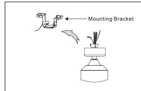
3-1. Lift fan assembly onto mounting bracket.
