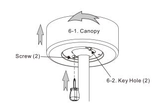
**Note:** Two screws are installed on mounting bracket for canopy installation.
