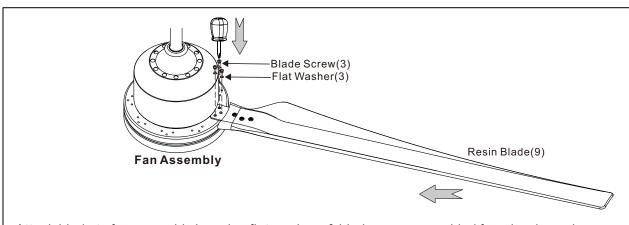
Attach blade to fan assembly by using flat washers & blade screws provided from hardware bag. (\* Repeat until all 9 blades are installed firmly.)
