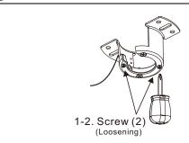
1-2. Loosen the screws at mounting bracket. **Do not remove.**
