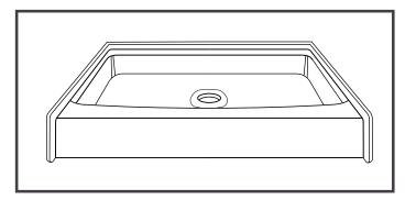
An opening in the slab or sub floor must be provided to permit the molded in drain boss to extend below the floor surface. The opening should be 5" x 5" minimum in size.
