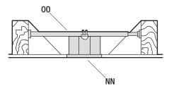
To hang your fan where there is an existing fixture but no ceiling joist, you may need an installation hanger bar (00) (not included) as shown above.
