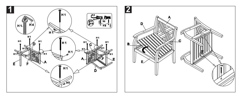
Step 1: attach right side (D) to the back (A). Then attach support L (E) and support S (F) to the right side (C) as shown on the picture by using the Allen Bolt (H1) and tighten with the Allen Key (H4). Continue with the left side (C) in the same way. Make sure to tighten all bolts (H1) before you continue with step 2. Step 2: put the seat (B) inside the chair as shown on the picture and use the screws (H2) to attach it to the chair by using a screwdriver .
