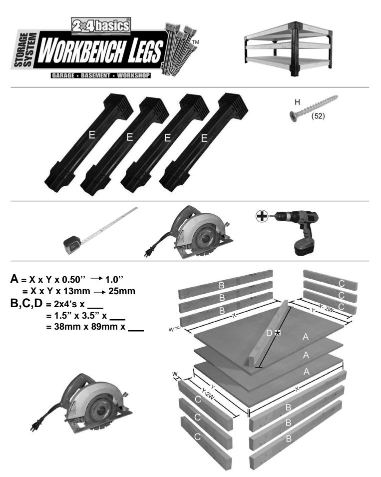
\* This diagonally placed 2x4 helps support the worktop. It is best cut to fit, but the length can be calculated as:
