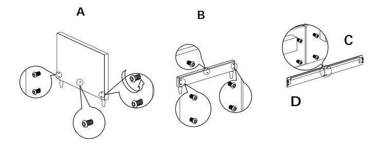
5. Attach middle metal support(G) to headboard(A) and footboard(B) with screws.
