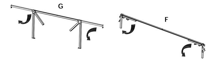
3.Put middle metal support(G) and horizontal metal support(F) together with screws(AA) by allen key(BB).
