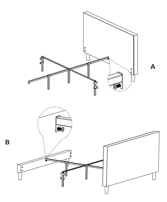
6.Put right bed frame(C) and left bed frame(D) to the brackets of horizontal metal support(F) and tighten the screws.
