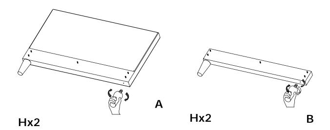
2. Open middle metal support(G) and horizontal metal support(F).
