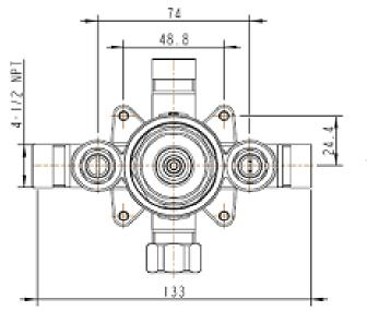
Pressure balanced tub and shower valve. Brass body.
