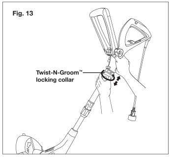
To convert your edger back to a trimmer, hold the handle, slide the Twist-N-Groom<sup>™</sup> locking collar downward and twist the handle counterclockwise while holding the pole to adjust the trimmer head to an angle of 0°. Ensure the locking collar snaps into place (Fig. 13).
