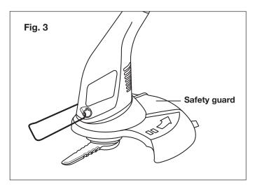
If needed, you can flip up the steel edger guide + flower guard onto the motor cover. This will allow you maximum use of the SharperBlade<sup>™</sup>.
