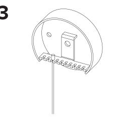
Once the base is installed, place the tool cables in the slots, and fasten the cap with the provided 3/8" tamper-resistant bolt.
