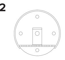
There are 4 mounting holes; only 2 need to be used. For installations into a vertical stud, use the 2 vertically oriented holes. The horizontally oriented holes can be used for other types of installation. 3/8" wedge anchors, lag bolts, or other fasteners may be used.
