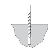
Drill the holes in accordance with the specifications shipped with the anchors. Make sure the holes are at least 3" away from any cracks in the base material.
